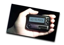
**SwimGuard Edge** simulates the scanning procedures of a lifeguard which includes continuous headcounts. All swimmers are monitored simultaneously and if a person requires assitance, an alert is delivered via a pageing system generated within 15 seconds giving ample time for a responder to provide assistance.
